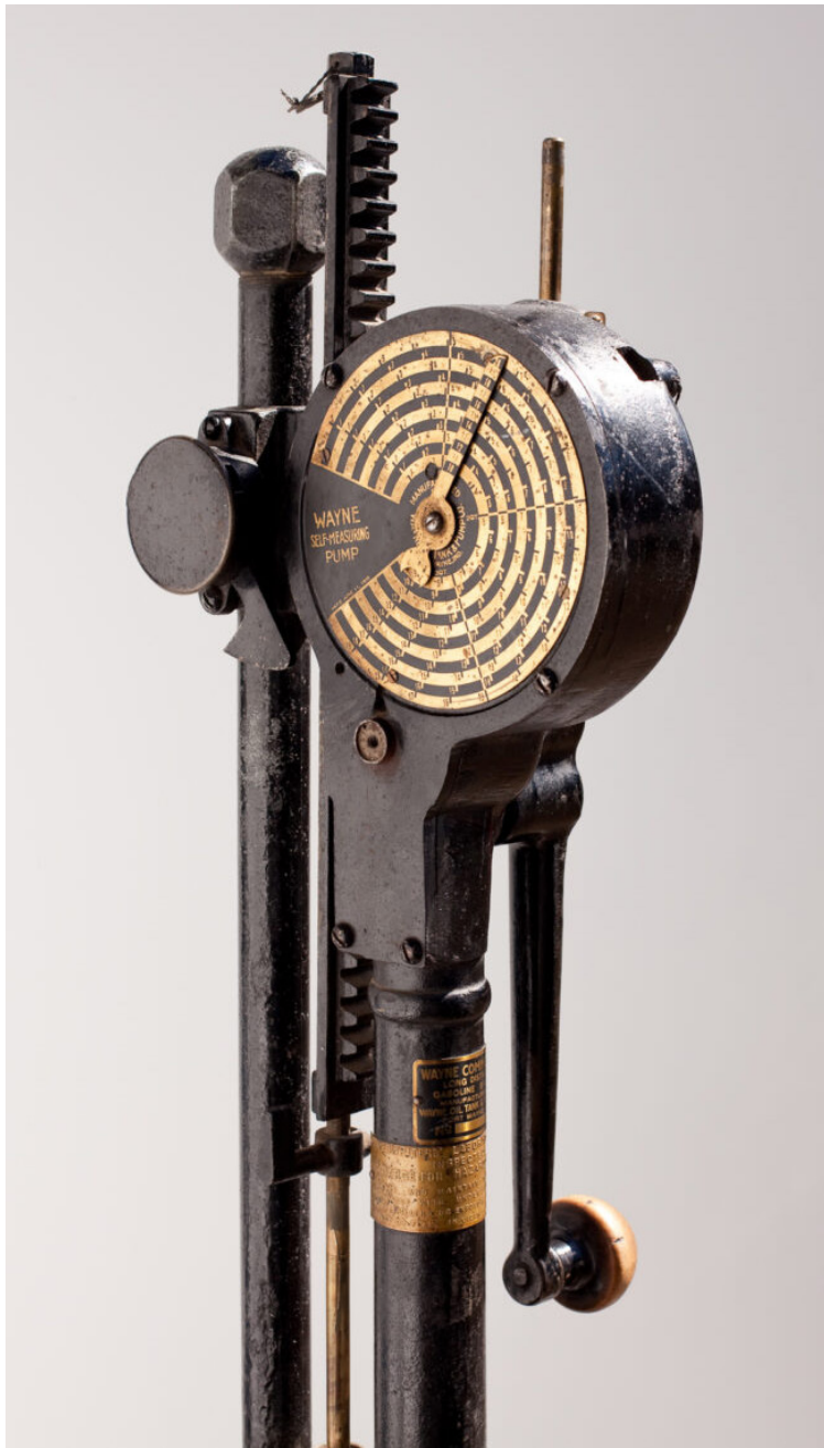
Detailed Wayne pump measurement scale 70 designed for dispensing kerosene and later, gasoline.
